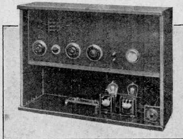
Fig. 1.—Central receiving set serving a group of schools through G.P.O. telephone lines. The line amplifier occupies the lower compartment of the cabinet.
